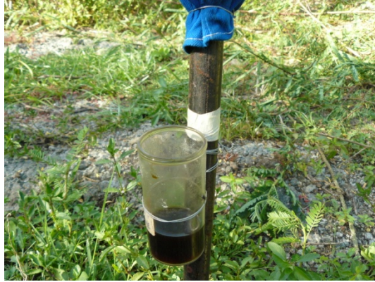
Figure 3: Urine Sample and Tape Wound Around the Base of the Biconical Trap
