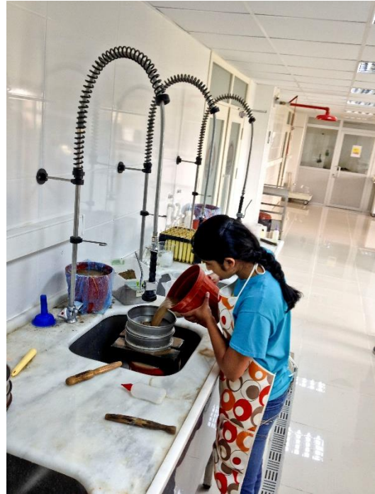
Figure 3: Washing soil samples to collect cereal cyst nematodes using the floatation method. (Picture Credit: Sevil Hanım)
