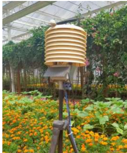
Fig. 3 three-in-one sensor for temperature, humidity and illumination of weather environment
